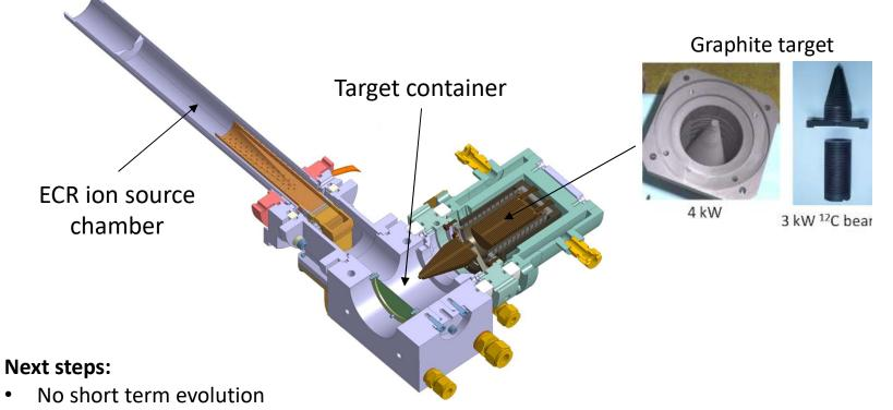
• But the ECR ion source could be connected to a small target cavity (TULIP type) to produce neutron deficient isotopes of Xe
