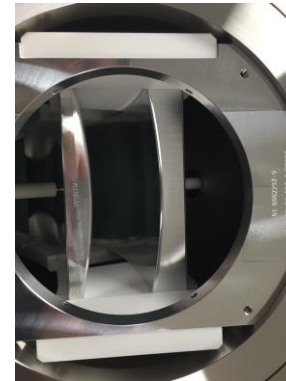
45°, 90° and 10° electrostatic deflector during FAT in 01/2020 at PFEIFFER
