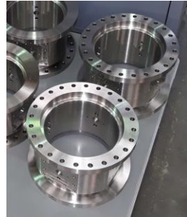
Electrostatic steerers during fabrication in 10/2019 at SOMINEX
