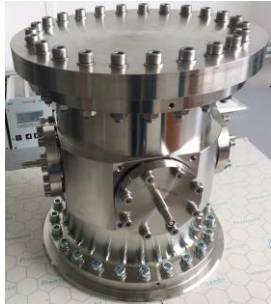
Electrostatic quadrupole during vacuum test in 04/2019 at VATEC
