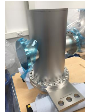
45°, 90° and 10° electrostatic deflector during FAT in 01/2020 at PFEIFFER
