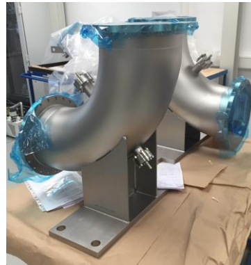
45°, 90° and 10° electrostatic deflector during FAT in 01/2020 at PFEIFFER
