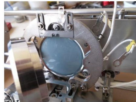
Side view: MCP + Phosphore screen
